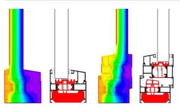
Metal Technology can provide tailored U-value calculations using their dedicated estimating software to calculate overall project average window U-values for their full range of systems.
