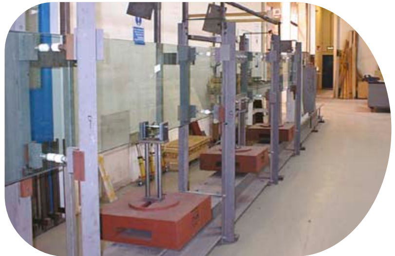
Glass Fin testing, Pilkington R&D Centre, UK.
